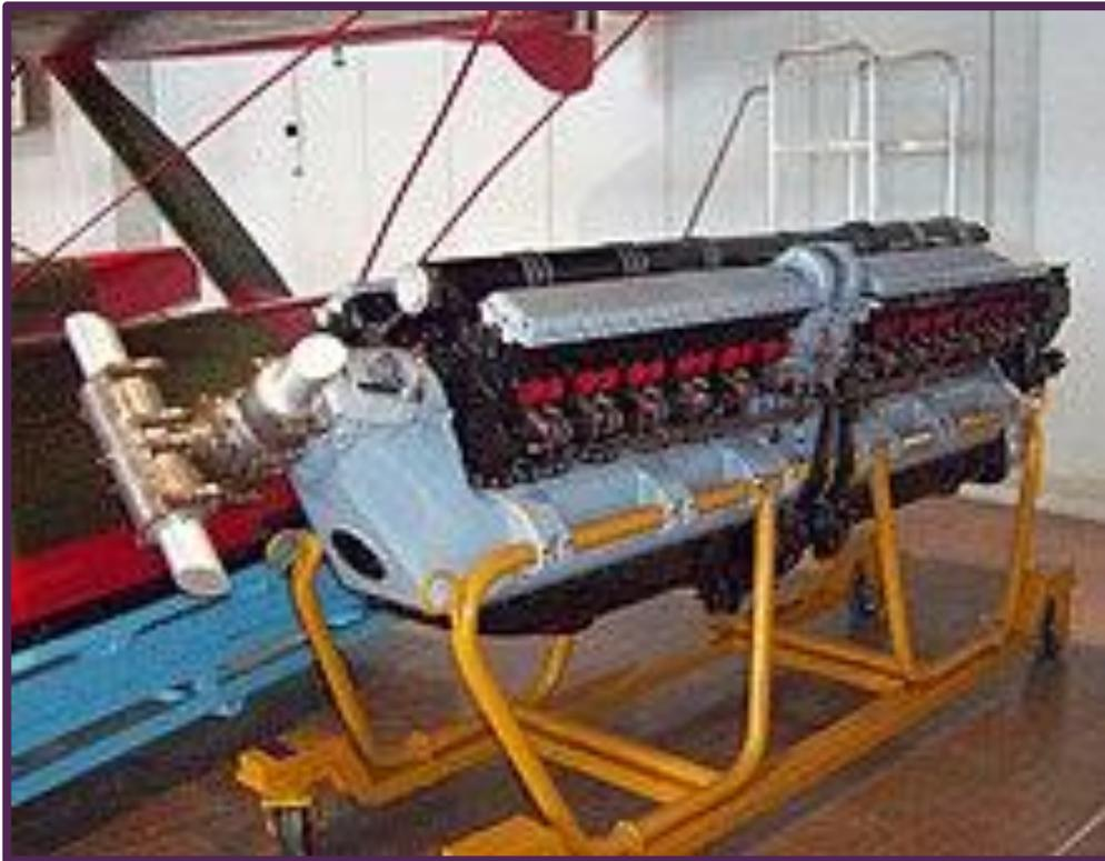
*Built by putting two V12 engines back to back, this motor was used to break the speed record for seaplanes. Read more about it on page 8. As a comparison, check out the history of the good 'ol Briggs and Stratton flathead "lawn mower" engine. Almost exactly the same engine as this one above, but with 1/24 the number of pistons.*
