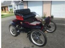
Tiller steering-hand clutch and throttle, foot brake, 2 forward and 1 reverse transmission, 8 horse power Briggs and Stratton, 2 brass coal oil lamps
